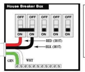
Important: Installation of this GFCI Circuit Breaker, including Ampere sizing and selection of conductor size and type, must be performed by a qualified electrician in accordance with the National Electrical Code, or the Canadian Electrical Code, and all federal, state, and local codes and regulations in effect at the time of installation.
